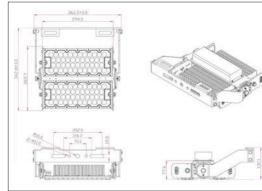
**LEDX PHOENIX 1** 240 watts including power adapter and power adapter box
